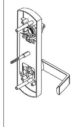
2. Place and fasten cam piece with locked type washer and screw
